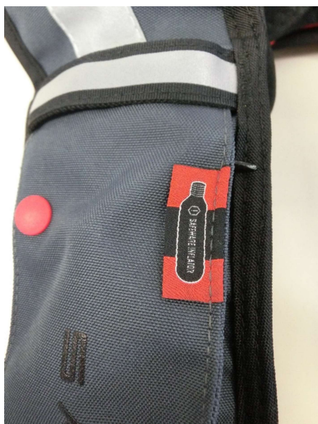
Pocket of the chartridge and triggering system
